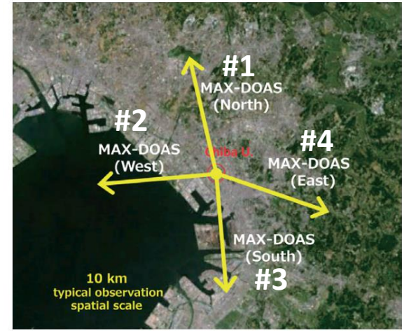
Fig. 5 Schematic illustration of observations by the North-, West-, East-, and South-viewing MAX-DOAS instruments (this set is called the 4AZ-MAXDOAS system) located at the SKYNET Chiba site (Chiba University).
